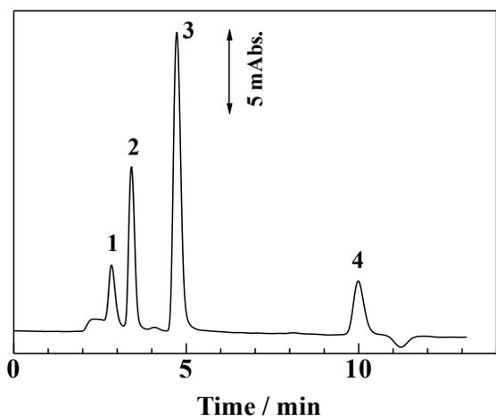
Fig. 5 Separation of UV-absorbing anions on a C30 column permanently coated with PEG-20000. Eluent, 300 mM sodium sulfate; analytes, iodate (1), nitrate (2), iodide (3), thiocyanate (4); analyte concentration, 0.2 mM each; other operating conditions as in Fig. 3. Reproduced from Ref. 14 with permission.
