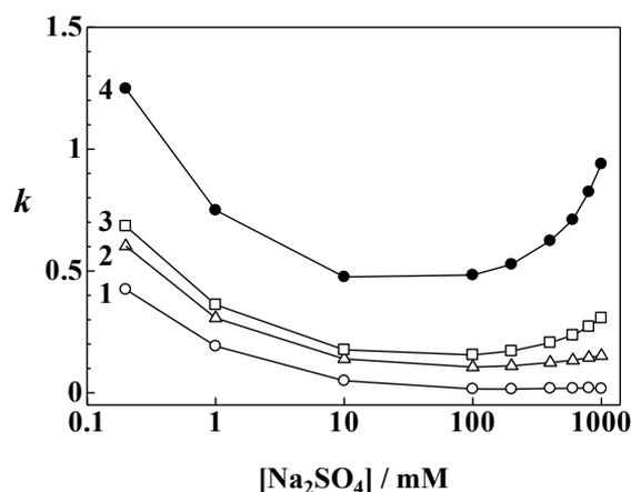
Fig. 9 Retention factor of analytes as a function of sodium sulfate concentration. Operating conditions as in Fig. 8. Reproduced from Ref. 12 with permission.
