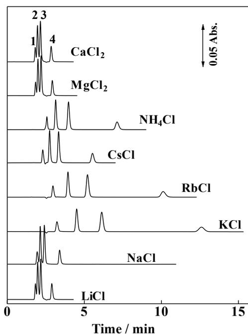
Fig. 16 Separation of inorganic anions on a C30 column using eluents containing different cations. Column, Develosil C30-UG-5 (100 × 0.53 mm i.d.); eluents, 10 mM chloride containing 0.1% (w/v) 18C6 and 3% (v/v) acetonitrile; flow rate, 8.0 μl/min; wavelength of UV detection, 210 nm; analytes, 0.2 mM each of iodate (1), nitrate (2), iodide (3) and thiocyanate (4); injection volume, 0.15 μl. Reproduced from Ref. 19 with permission.
