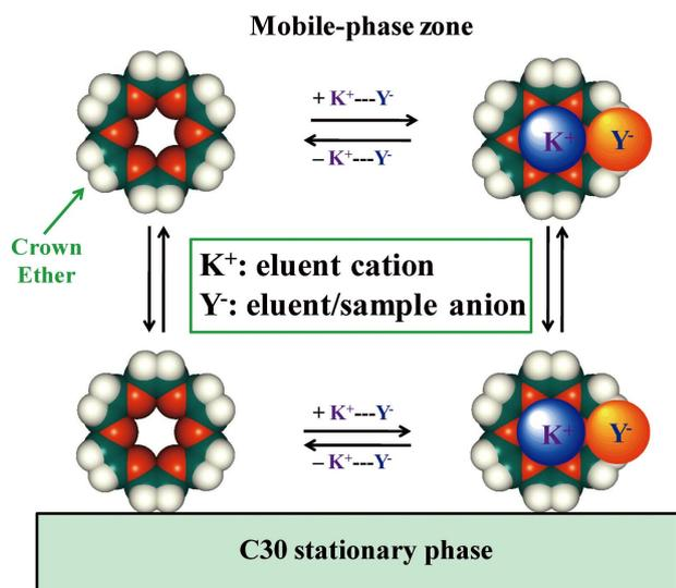
Fig. 15 Retention mechanism of 18C6 and ions. Adapted from Ref. 19 with permission.
