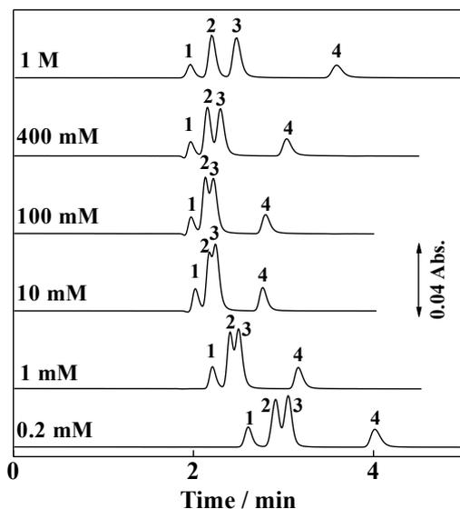
Fig. 8 Separation of anions on an unmodified C30 column using different concentrations of sodium sulfate as the eluent. Column, Develosil C30-UG-5 (C30), 100 × 0.53 mm i.d.; eluent, sodium sulfate, the concentrations as indicated; flow-rate, 8.0 μl/min; analytes, iodate (1), nitrate (2), iodide (3), thiocyanate (4); concentration of analytes, 0.1 mM each; injection volume, 0.15 μl; wavelength of UV detection, 210 nm.
