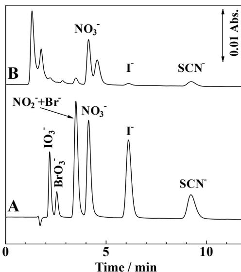
Fig. 12 Separation of inorganic anions in saliva on a Methyl-12OE-bonded stationary phase. Column, Methyl-12OE (100 × 0.53 mm i.d.); mobile phase, 50 mM sodium sulfate; flow rate, 8.0 μl/min; wavelength of UV detection, 210 nm; samples, 0.2 mM each of iodate, bromate, nitrite, bromide, nitrate, iodide and thiocyanate (A), saliva sample (B); injection volume, 0.15 μl. Reproduced from Ref. 17 with permission.
