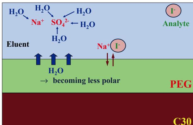
Fig. 4 Description of PEG stationary phase and interaction between analytes and PEG phase.
