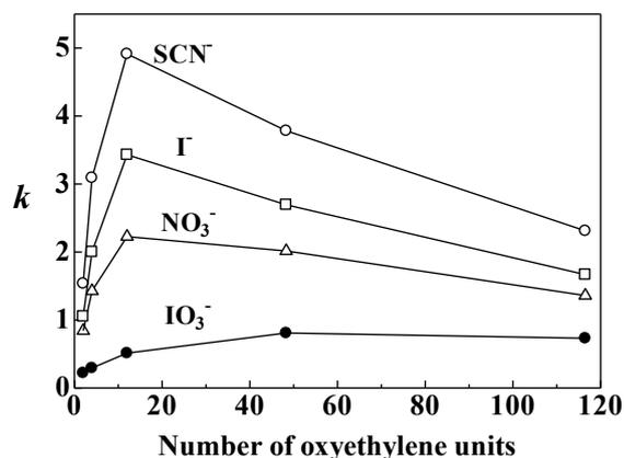
Fig. 13 The retention factor as a function of oxyethylene unit number. Columns,  $100 \times 0.53$  mm i.d.; mobile phase, 50 mM sodium sulfate; flow rate,  $8.0 \mu\text{l}/\text{min}$ ; wavelength of UV detection, 210 nm; analytes, 0.1 mM each; injection volume, 0.15  $\mu\text{l}$ . Reproduced from Ref. 17 with permission.
