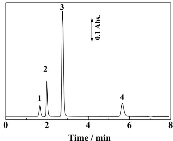
Fig. 6 Separation of UV-absorbing anions on a conventional-size C30 column permanently coated with PEG. Column, Develosil C30-UG-5 column ( $150 \times 4.6$  mm i.d.) permanently coated with 5% PEG-20000; eluent, 300 mM sodium sulfate and 50 mM sodium chloride; flow-rate, 1.0 ml/min; injection volume, 20  $\mu$ l; analytes, iodate (1), nitrate (2), iodide (3), thiocyanate (4); analyte concentration, 0.2 mM each; wavelength of UV detection, 220 nm. Reproduced from Ref. 15 with permission.
