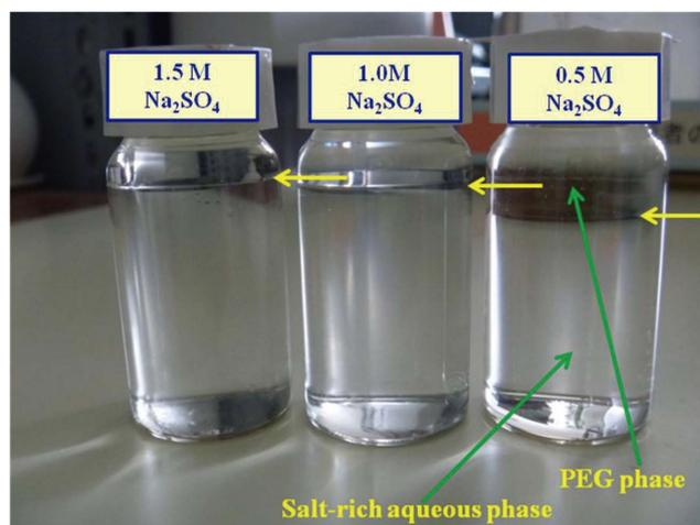
Fig. 2 Effect of sodium sulfate solution on the PEG-phase volume. PEG-20000 (1 g) dissolved in 19-ml volume of different concentrations of sodium sulfate solution.
