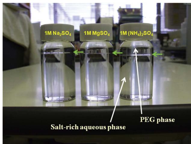
Fig. 1 Phase separation for PEG and aqueous sulfate solution. PEG-20000 (1 g) dissolved in 19-ml volume of 1 M each sulfate solution.
