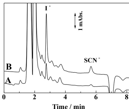
Fig. 7 Separation of iodide and thiocyanate in seawater sample. Samples: lower trace (A), 20  $\mu$ l seawater; upper trace (B), seawater spiked with 254 ng/ml iodide and 58 ng/ml thiocyanate. Other operating conditions as in Fig. 6. Reproduced from Ref. 15 with permission.
