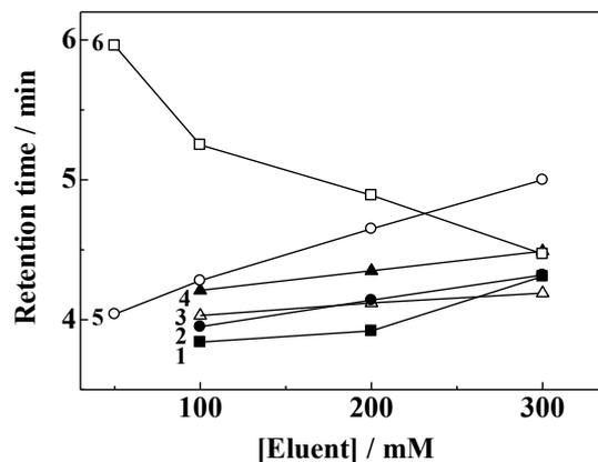
Fig. 3 Retention time of iodide as a function of the eluent concentration. Column, Develosil C30-UG-5 (100  $\times$  0.32 mm i.d.) modified with 5% PEG-20000; eluent, magnesium sulfate (1), potassium chloride (2), sodium chloride (3), lithium chloride (4), sodium sulfate (5), ammonium sulfate (6); flow-rate, 2.1  $\mu\text{l}/\text{min}$ ; injection volume, 0.2  $\mu\text{l}$ ; analyte, 1 mM iodide; wavelength of UV detection, 220 nm. Reproduced from Ref. 14 with permission.
