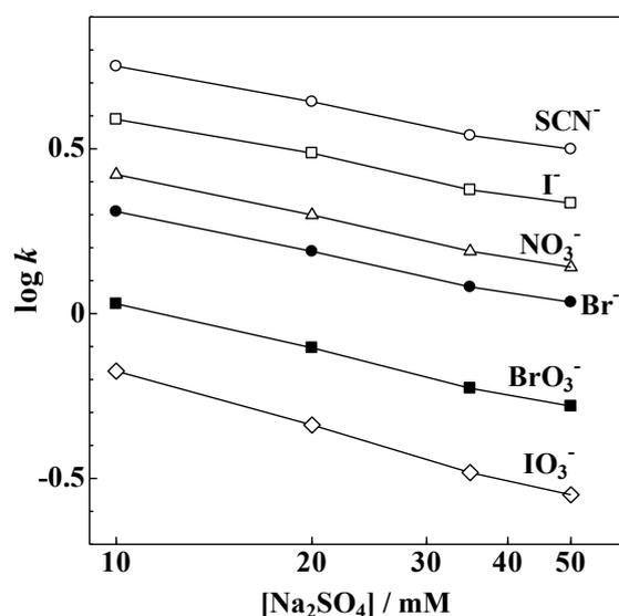
Fig. 11 Effect of sodium sulfate concentration on the retention of analyte anions. Column, Methyl-12OE, 100 × 0.53 mm i.d.; eluent, sodium sulfate; flow rate, 8.0 μl/min; analyte concentration, 0.2 mM each; injection volume, 0.15 μl; wavelength of UV detection, 210 nm. Reproduced from Ref. 16 with permission.
