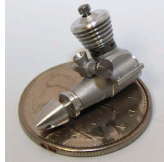
Ronald Valentine Engines Nano Bee 0.006 (Diesel type) Bore 2.0 mm Stroke 2.0 mm Rpm 16,200 rpm Displacement 0.006 cc Air flow rate 97.2 sccm Thermal efficiency ???
