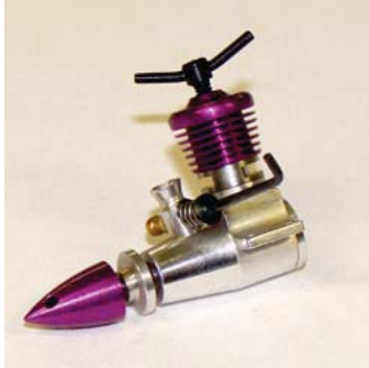
Ronald Valentine Engines Mini Bee 0.021 Mk II (Diesel type) Bore 3.0 mm Stroke 3.0 mm Rpm 16,200 rpm Displacement 0.021 cc Air flow rate 340 sccm Thermal efficiency ???
